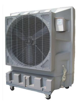
The arrangement of the components is shown in fig. there is a separate motor for the pump and fan so they can be used independently. The arrangement of the components in a box providing 3 pads. The pump , pumps the water from the bottom tank to the top and water trinkles through the holes provided on the top of tank and falls passing the pads to the bottom tank.
